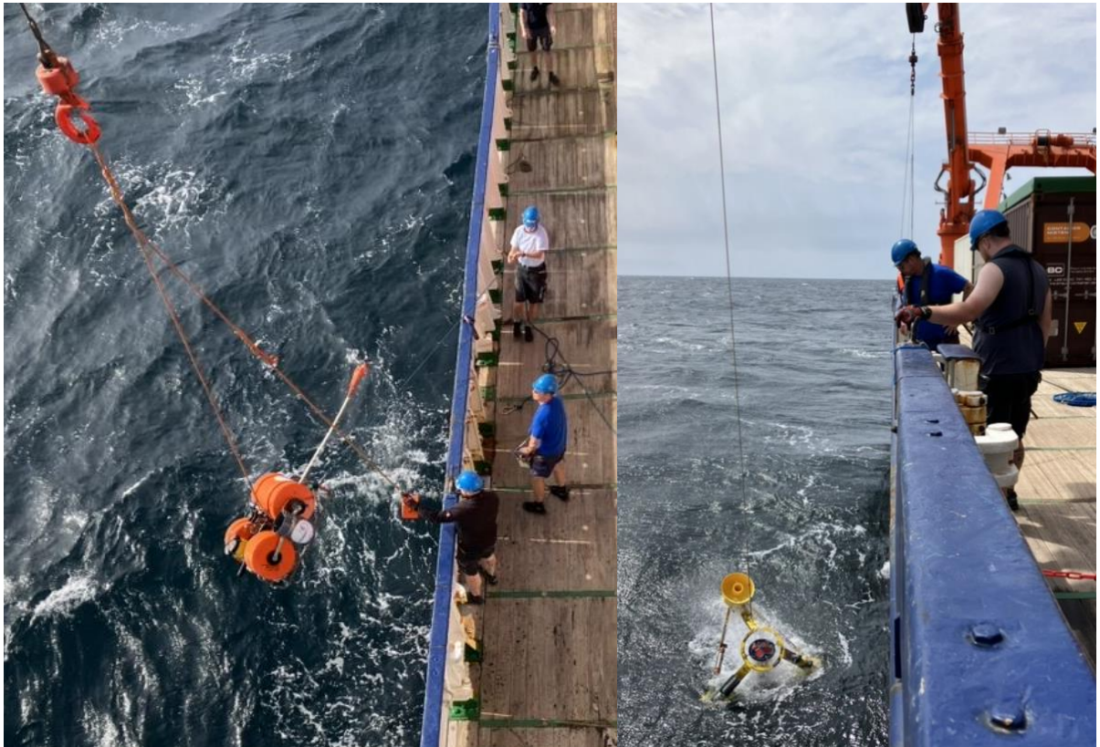
Fig. 2: Recovery of the lander equipped with an acoustic Doppler current profiler (ADCP) and a SUNA nitrate sensor (left), and the tripod with an ADCP. The moorings were deployed at depths of 100 m and 50 m, respectively, to capture internal waves propagating toward the coast (Photos: Peter Brandt).
