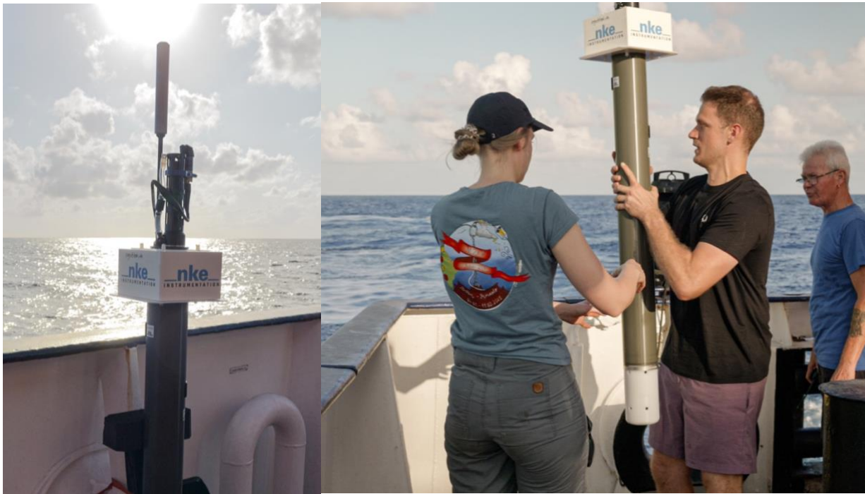
Fig.4: Left: Argo Float with temperature, salinity and oxygen sensors. The white antenna can be seen at the top. Right: Argo Float being deployed over the stern of FS Meteor. Photos: David Menzel.
