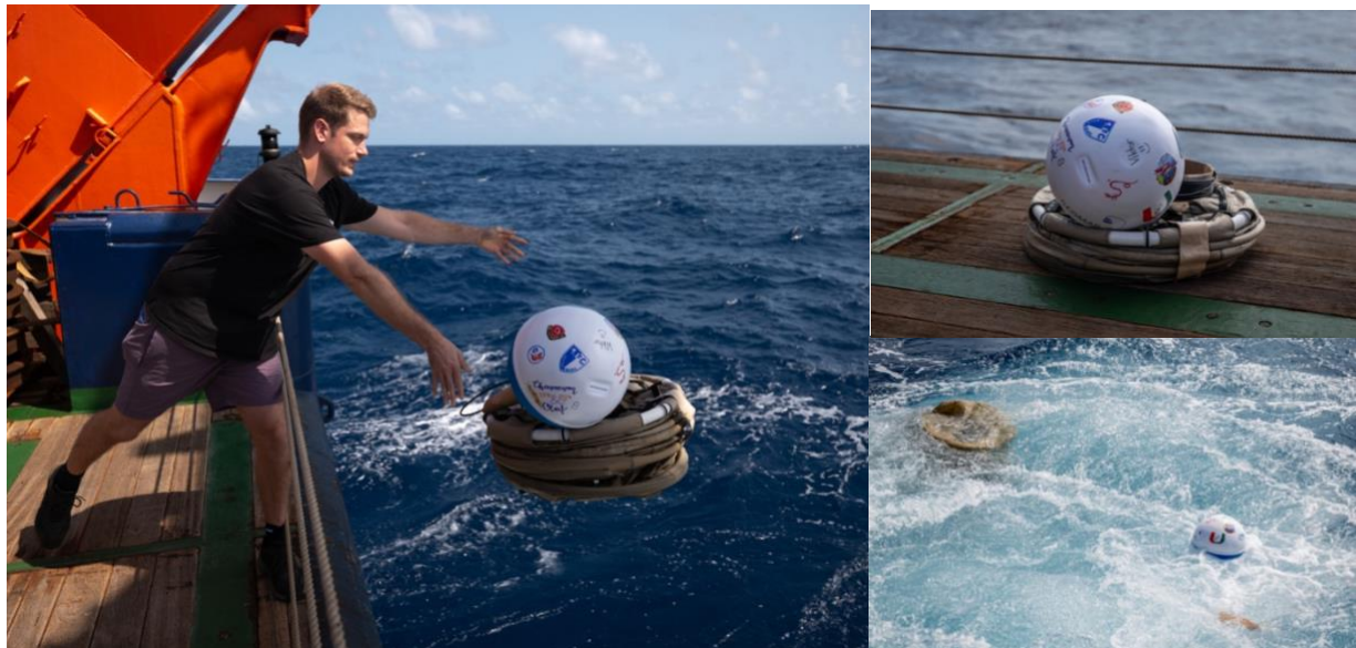
Fig.3: Deployment of an SVP surface drifter over the stern of FS Meteor. Photos: David Menzel.
