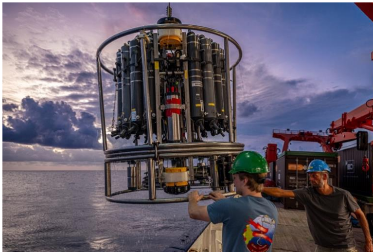
Fig. 2: Deployment of the CTD probe at dusk. The actual CTD is located at the bottom of the CTD rosette. Above it one can see the water samplers arranged in a circle and in the foreground the two yellow lowered ADCPs, one of which 'looks' upwards and the other downwards. Photo: David Menzel.
