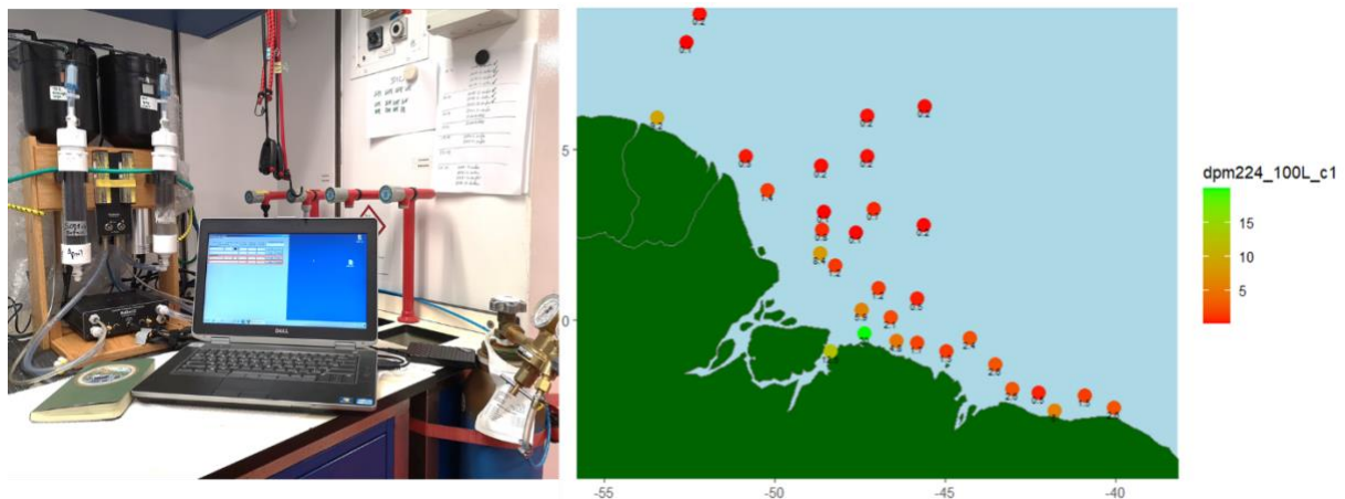
Fig. 4: RaDeCC measuring device with control computer and helium supply (left). Preliminary results of the ^{224}\text{Ra} measurements in the working area show different signatures for the different coastal regions and the open seawater (right; photo and graphics: David Kaiser).
