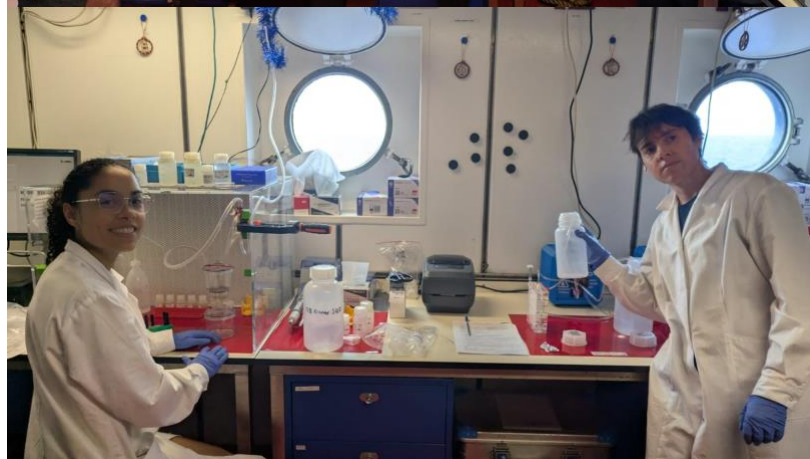
Fig. 2b: Laboratory for the filtration of water samples for later trace metal analysis in different size fractions between truly dissolved and particulate: Sequential filtration through membrane filters (Caitlyn Kelly, left) and ultrafiltration (Adrian Hollister, right).
