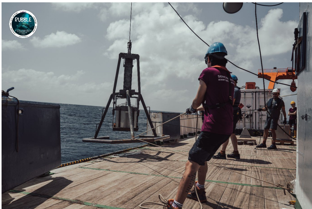
Figure 3. Box Corer (BC) deployment from RV METEOR during its 205 th voyage, the “RUBBLE” expedition.
