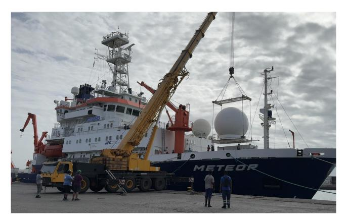
The SEA-POL radar antenna is installed on the forecastle deck of FS METEOR in the port of Mindelo.
