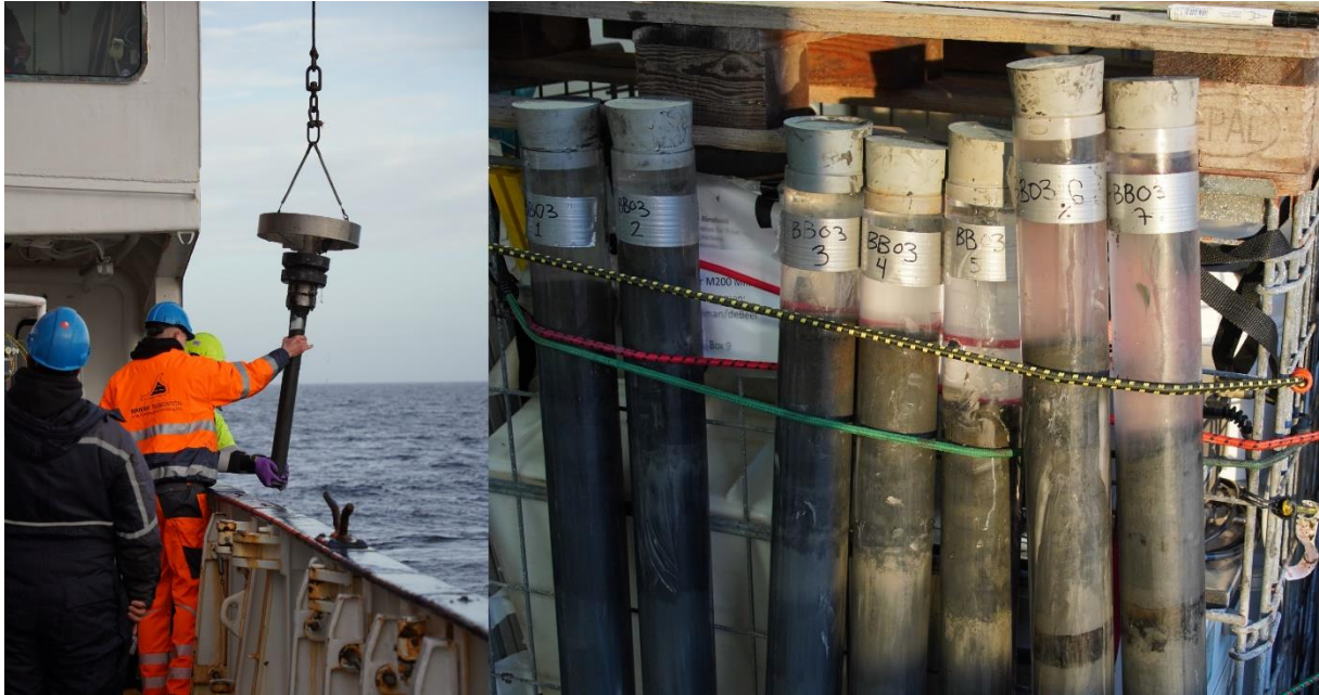
Obtaining surface sediment samples with the Rumohr corer in the Bornholm Basin (photo: V. Mohrholz)
