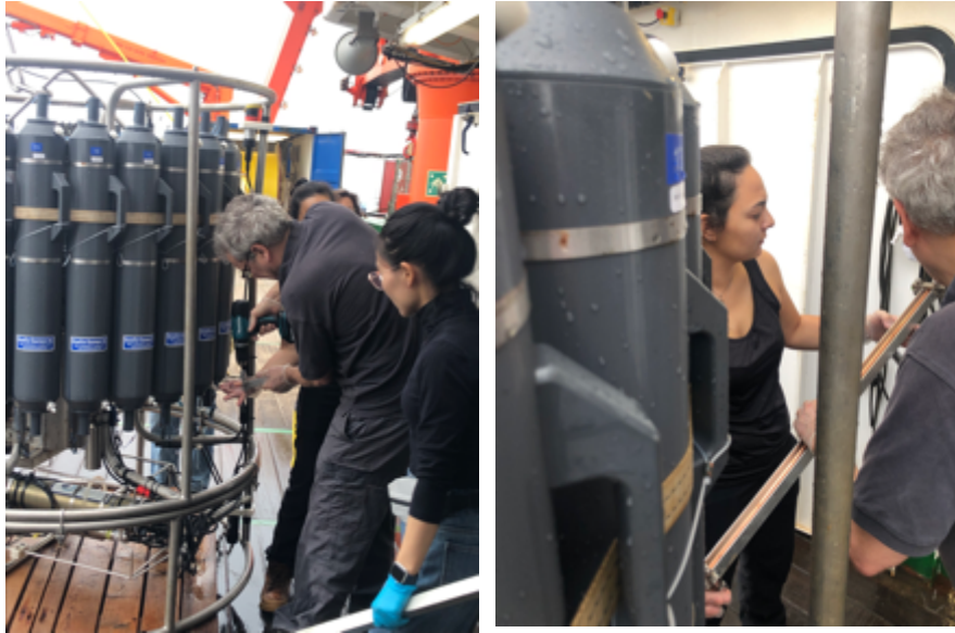
Figure 2. Collecting samples for helium-3 analysis in copper tubes at the Napoli mud volcano station.
