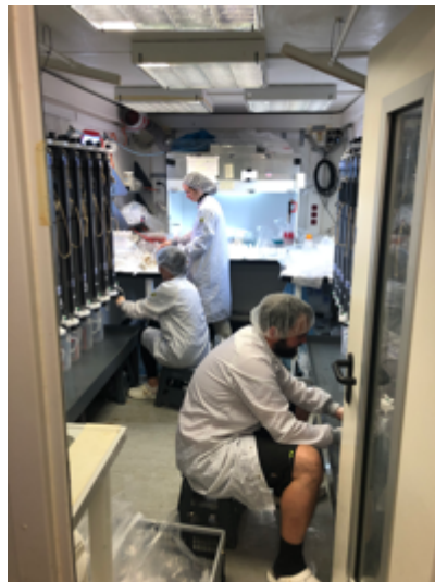
Figure 1. Left: Sampling for trace metal concentrations in seawater using a titanium-frame CTD and winch with Kevlar cable (yellow). Right: Sampling from the trace metal CTD bottles inside a dedicated sampling container (white container at the aft of the ship in the photo on the left).
