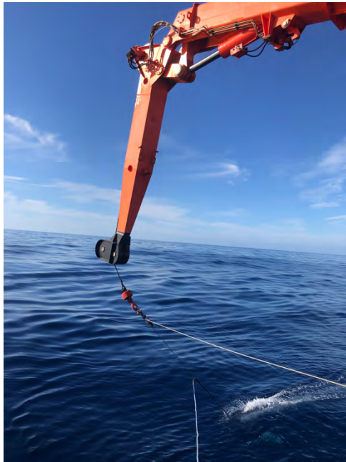
Figure 2. The so-called 'tow-fish', which is used to pump seawater into a laboratory on RV Meteor. This water is uncontaminated with trace elements and can be used for experiments to test the controls on phytoplankton growth in this region.
