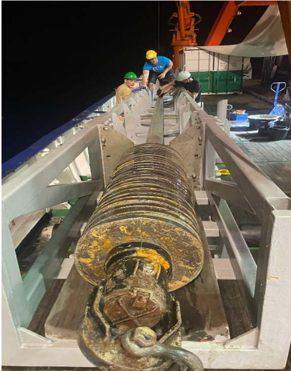
Figure 2: Preparation of the 18 m gravity core, comprised of three 6 m segments. (Foto: M. Stuhr).
