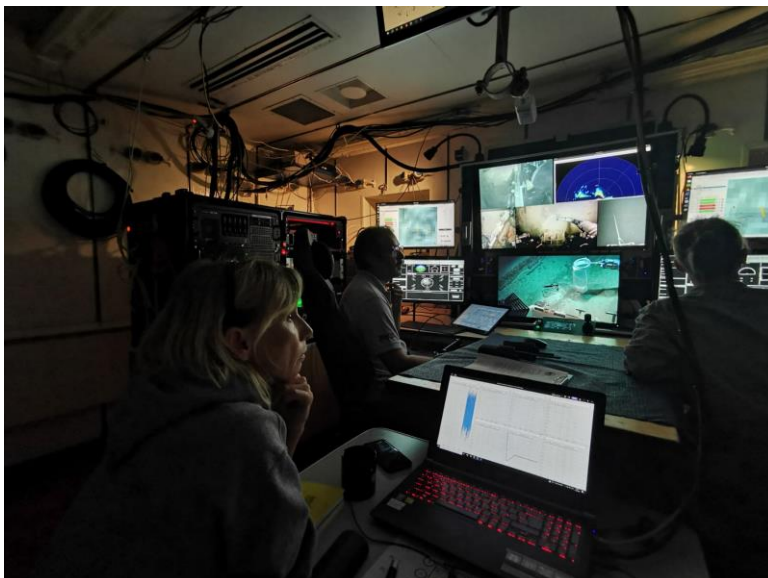
Figure 3: Control center of the ROV with two pilots and two scientists accompanying the dive. During the dive, which lasts about 6 hours in total, they work in shifts. (Foto: M. Taviani).
