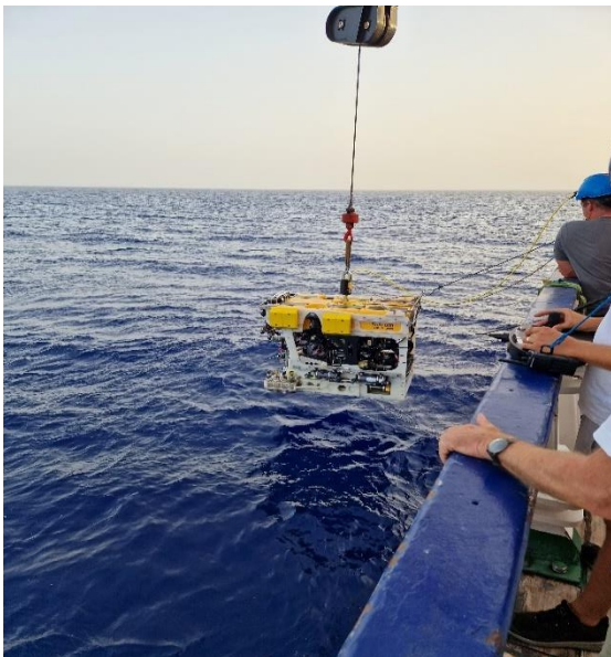
Figure. 3: The MARUM Squid ROV during the preparation for a dive mission. Before each dive, which takes about 6-8 hours, all systems and functions of the ROV are thoroughly checked by the four-member ROV team. (Foto: T. Lüdmann).
