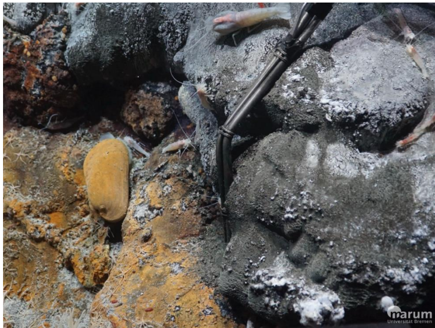
Fig. 1: Warm waters, which we prefer to sample at M190, emerge from under a hydrothermally formed crust (right). The suction port of the sampling system can be seen in the picture as well as a mussel, shrimps and tiny brittle stars.
