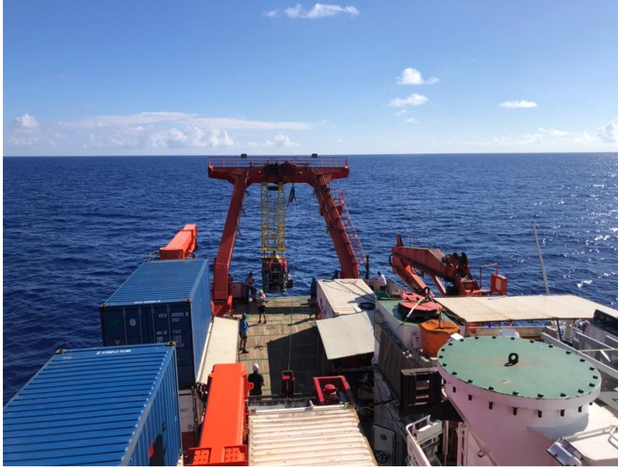
Fig. 3: The diving robot MARUM QUEST 4000 is deployed via the A-frame of FS Meteor. Even in the best weather and calm seas, this operation requires the highest concentration from the bridge, deck and ROV team. Foto: Christian Ostertag-Henning
