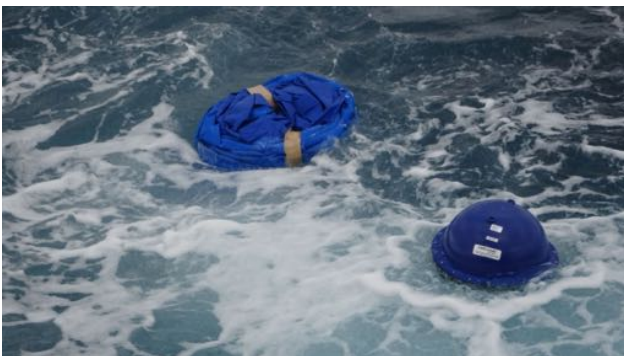
Fig. 4: The two types of drifters during deployed: SVP (Surface Velocity Project) drifter with a sail at 15 m depth on the left and a custom build hereon drifter on the right (Photos: A. Welsch).
