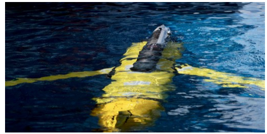
Glider during ballasting test (photos: C. Mertens).
