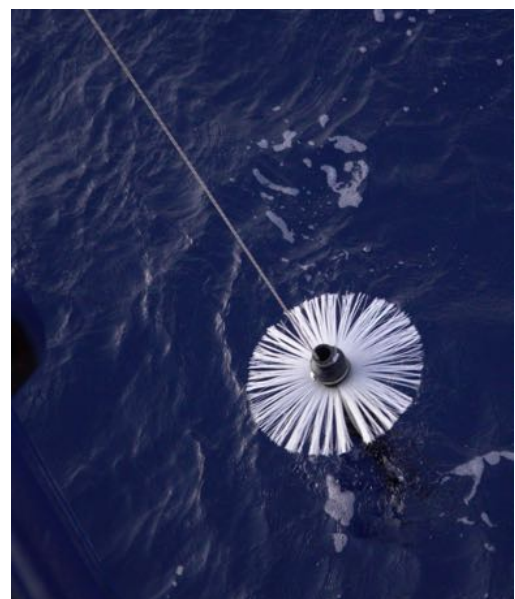
Fig. 2: First deployment of the microstructure profiler to measure turbulence in the upper ocean.
