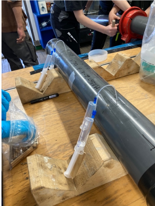
Fig.2 Left: Rhizone sampling of a sediment cores, photo: Sofia Ramalho Right: Rhizone sampling of a MUC core, photo: Johanna Schenk
