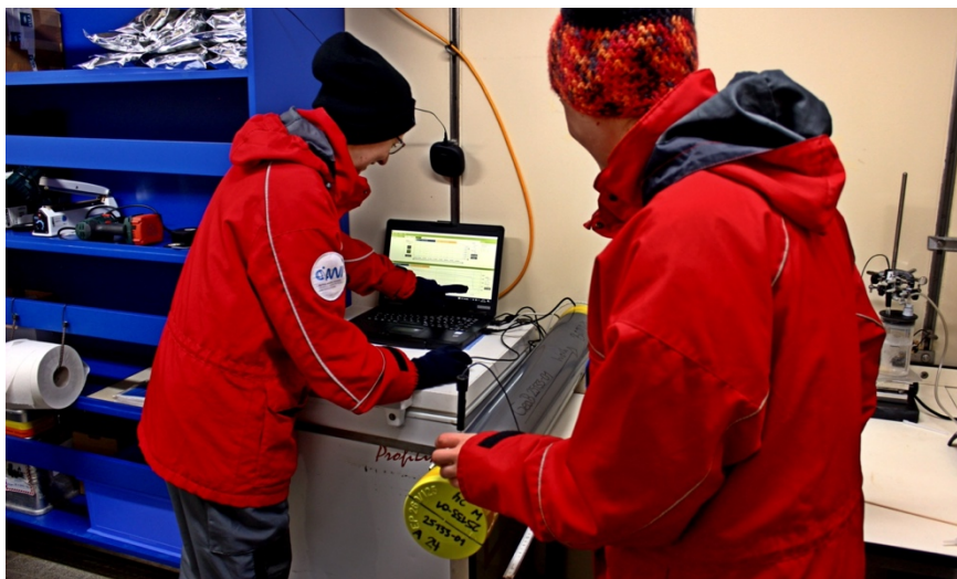
Fig. 3: Christina Nadolsky reads sensor signals that are used to calculate the oxygen concentrations. These measurements can take place over an entire night and take place at a cool 4°C. Kudos!
