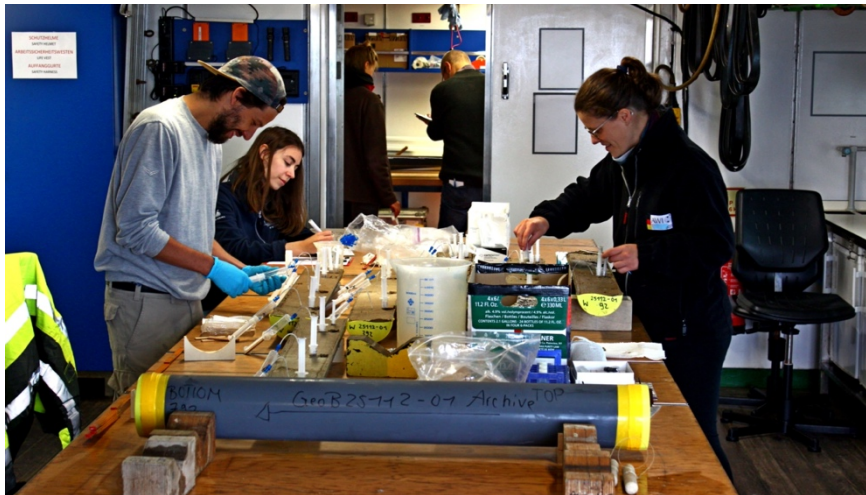
Fig. 2: In Meteor's geo-lab, Christopher Schmidt and Kim Moutard (left) sample sediment cores with Jessica Volz, which Aaron Roehler had previously sawn open professionally.
