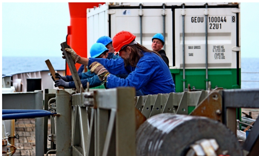
Fig. 3: With combined forces, a gravity corer is prepared in the core setting rack for the removal of the sediment core.
