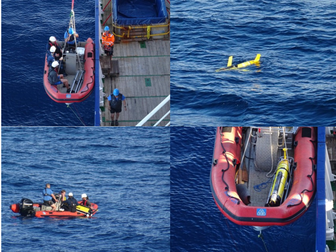
Sequence of glider recovery (clockwise): 1) Zodiac is lowered from the METEOR; 2) Glider in the water awaiting retrieval; 3) Glider being towed onto zodiac; 4) Zodiac with glider back at the of the Meteor. Photos: E. Breuning.
