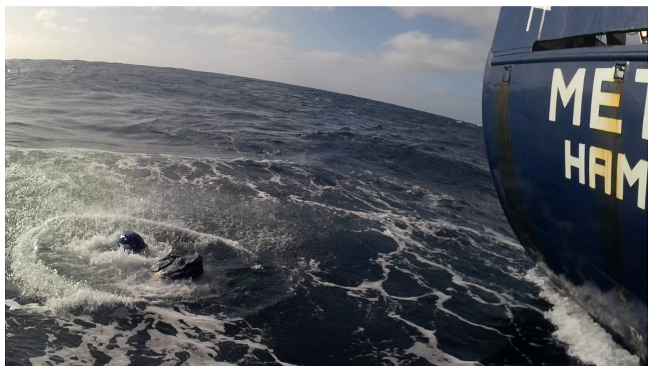
Two types of drifters after deployment: a small surface drifter manufactured by hereon (left), and the bigger SVP (Surface Velocities Project) drifter that has its drogue at 15 m water depth. Photos: J. Stake, H. Renzelmann.
