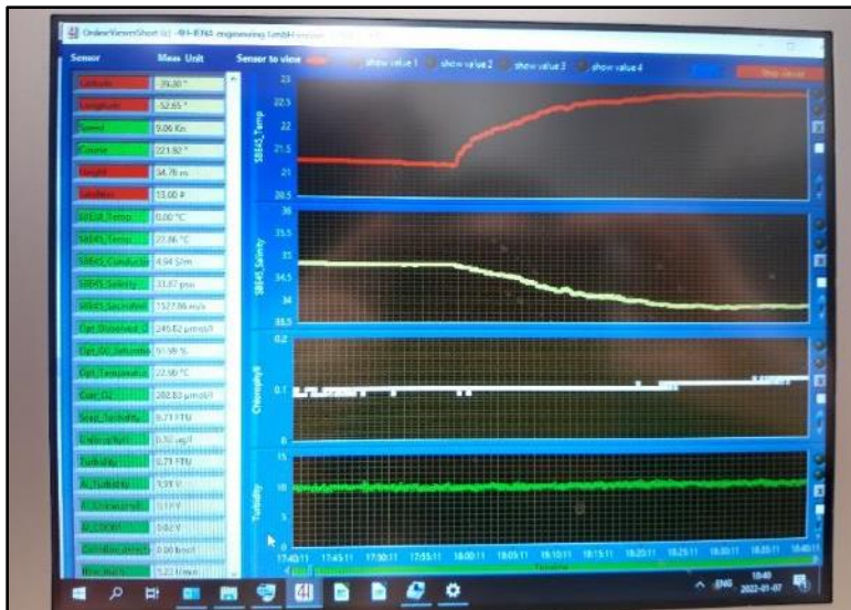
Fig. 2: Real-time data from the FerryBox when we passed the mouth of the Rio de la Plata (red: temperature, yellow: salinity, white: chlorophyll-a concentration, green: turbidity).
