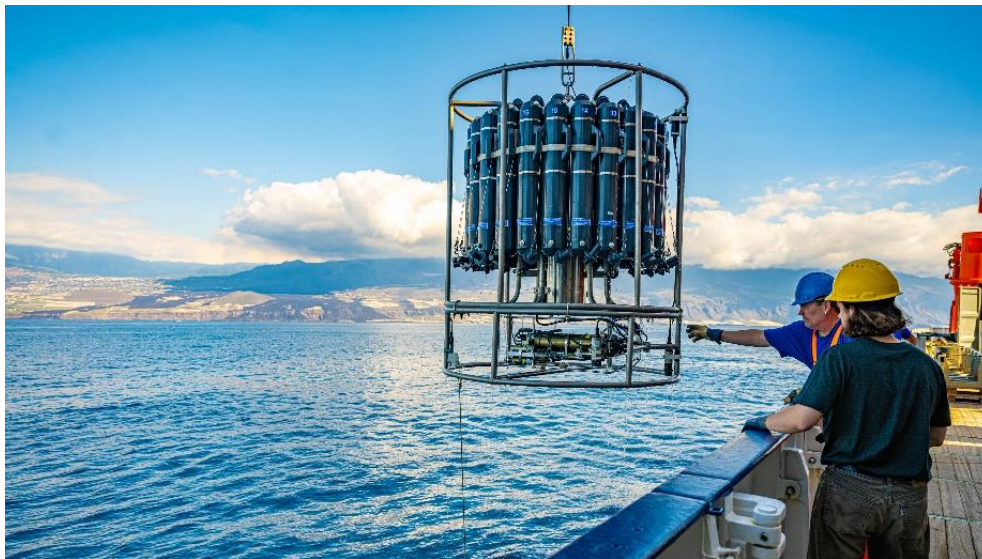
Photo 1: Deployment of the CTD rosette off the island of La Palma.
