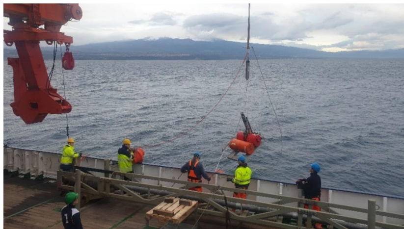
Photo 1: The deployment of a marine geodesy station offshore Etna (Photo: Alessandro Bonforte)
