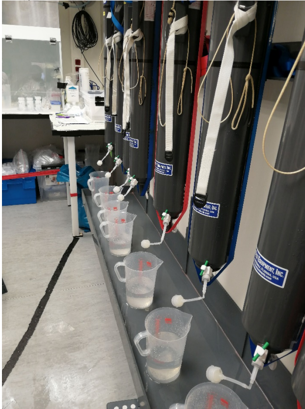
Fig. 3: Filtration set up in our clean container. (Photo: Linbin Zhou)
