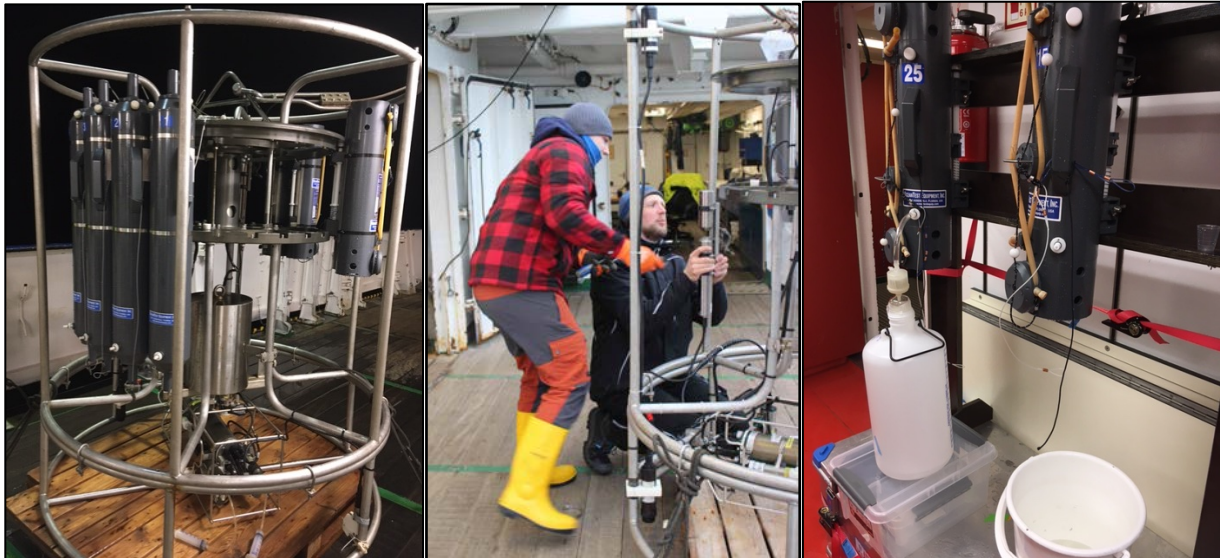
Photo left: CTD-rosette water sampler, our main working tool; center: David Ernst and Dennis Krämer prepare the CTD for the next deployment; right: The trace-metal clean GoFlo bottles in the lab for extraction of the water samples. (Photos by Adrienne Hollister (left, right) and Franziska Klimpel (center))
