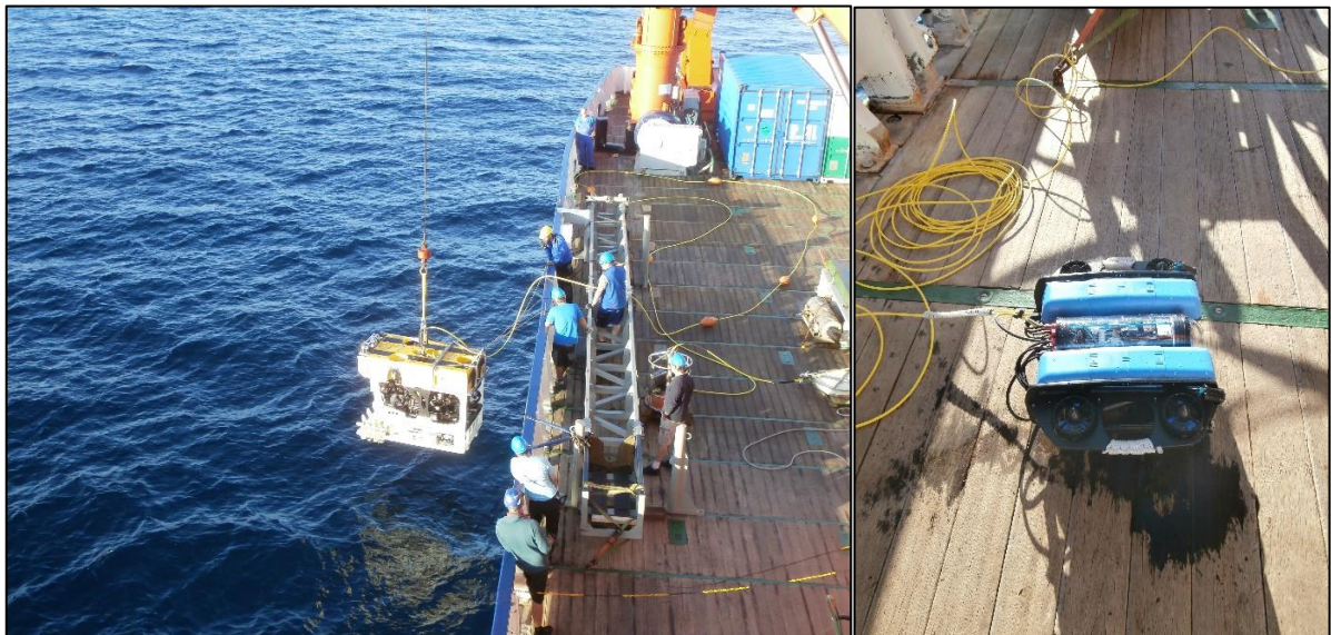
Figure 2: ROV SQUID being deployed, b) BlueROV resting on deck after deployment (Photo: W. Menapace)
