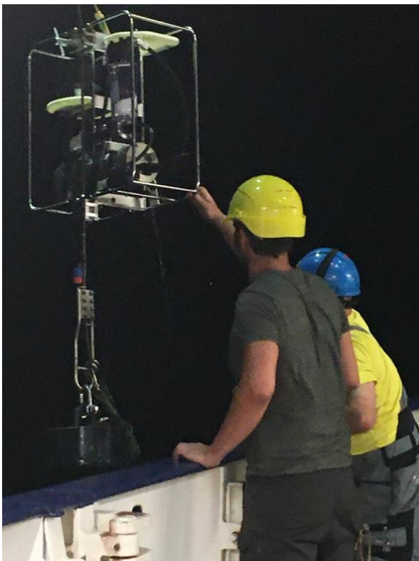
An in-situ pump is recovered.
