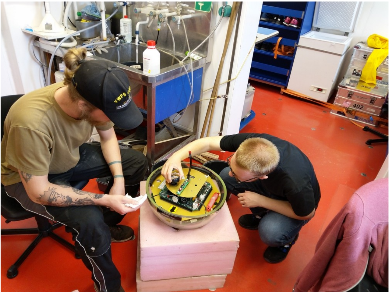
The inside of a PIES is inspected and checked for damage. Photo: K. Wiegand.
