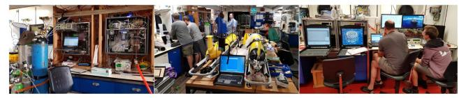
Lab scenes: Automatic system for measuring  $CO_2$  in surface water (left); gliders are being prepared for deployment in the geolab (center); the CTD watch is preparing for the next use of the CTD rosette system (right).
