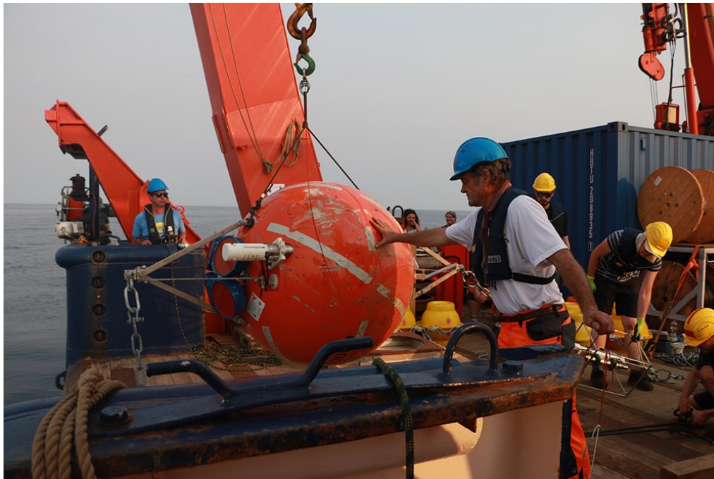
Fig. 2: Deployment of the current meter mooring off Angola from the stern of RV METEOR (Photo: Alba Filella Lopez de Lamadrid).
