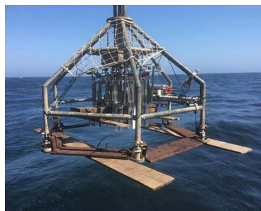
Fig.2: Multicorer with various wooden attachments that prevent the instrument from sinking too deeply but also ensure that it closes. (Photo: M. Zabel)
