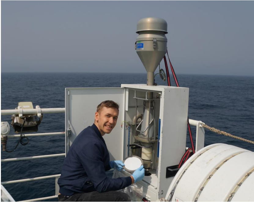
Figure 1: Marco Wietzoreck from MPI for Chemistry in Mainz exchanging the filter at the air sampler.
