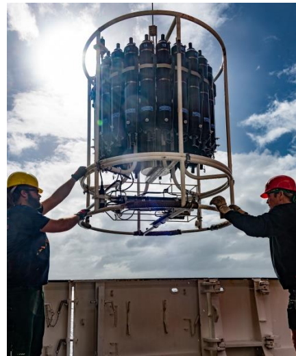
M151-2 deployment of the CTD with a lucky moment of sunshine
