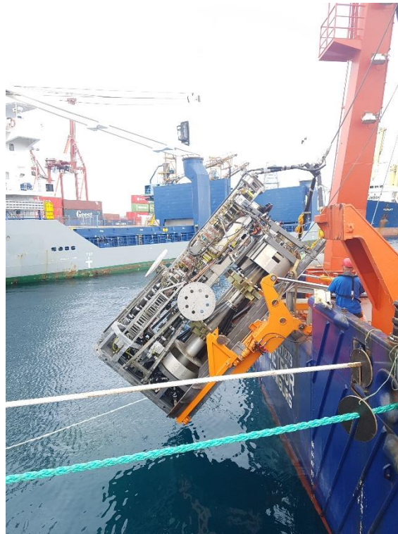
Abb. 2: Test of the seafloor drill rig MeBo in the port of Las Palmas. During the test import function were checked without deployment.
