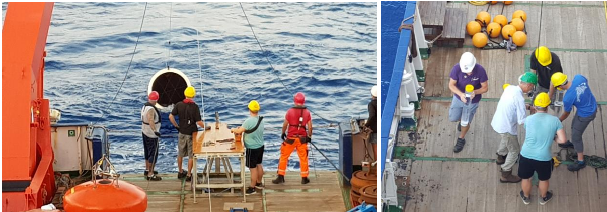
Left: the first sediment trap of the M3 mooring is taken on deck. Right: recovery of the sampling cylinders from the drifting sediment trap.
