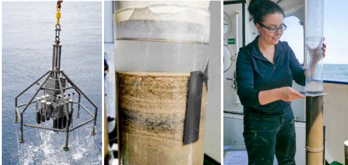
The multi corer returns full of sediment back on ship. The differently colored layers are archives of ocean changes off the past 1000 years..Right Dr. Sümeyya Eroglu cuts the core on 1cm thick slices.
