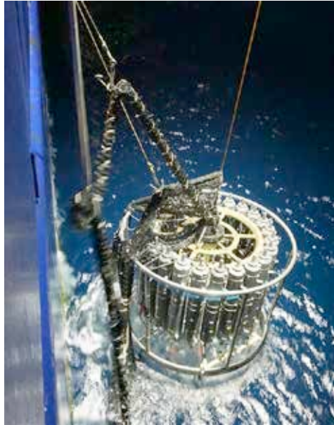
Fishernet entangled in the CTD and bow thruster of METEOR. (Foto: Sunke Schmidtko)
