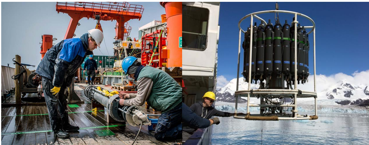
Fig. 1: After deployment in the Church Trough the autoclave gravity core DAPC is checked for sealage on deck of RV METEOR.
