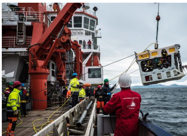
Figure 4: First deployment of MARUM ROV SQUID 2,000 m to study the shelf troughs (© vdL).
