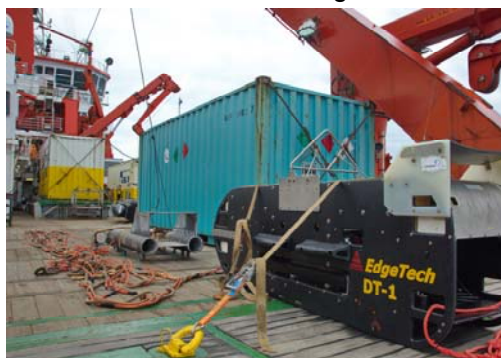
Figure 3: Configuration of the deep-towed sidescan sonar DTS-1 prior to deployment. The towfish is connected via umbilical to the 750 kg depressor weight.
