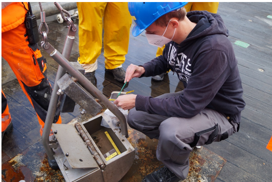
Figure 2: Sampling of the surface sediments at a sediment grab
