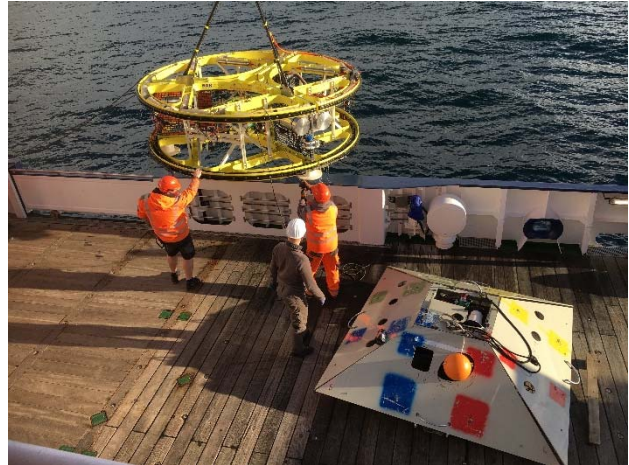
Figure 4: The Golden Eye (yellow) being launched to obtain electromagnetic information of the upper sediment layers. On deck is also the sonar lander, which was launched shortly afterwards on the seafloor to observe gas seeps over a period of several days. (© Yann Marcon).
