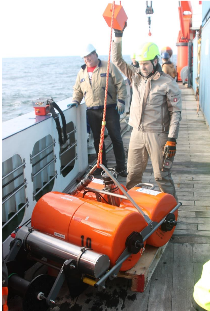
Fig. 2: Recovery of an ocean bottom seismometer (OBS). The devices are connected to the anchor weight with a coil and a rope (visible in the foreground of the OBS), which is subsequently recovered as well (photo S. Steuer).
