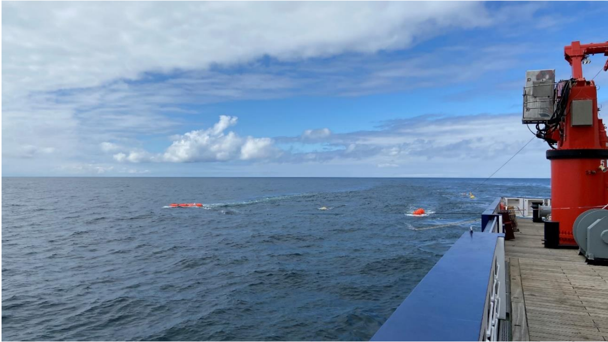
Fig. 2: View of the measuring equipment on the starboard side. On the outside you can see the paravan, further inside the yellow head buoy of the streamer cable, the orange buoyancy balls of the air pulsers and inside the yellow navigation buoy. Not visible here is the mirrored display of the measuring instruments on the port side.
