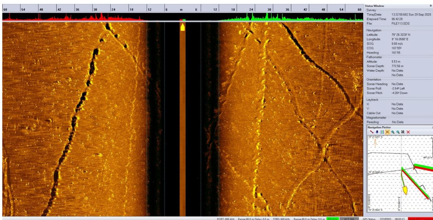
Raw sidescan data showing many trawl marks on the seafloor at 772 m depth, south west of Svalbard. Data collected by the PAUL 3000 Autonomous Underwater Vehicle.. RAW SIDESCAN PLOT: AWI AUV team
