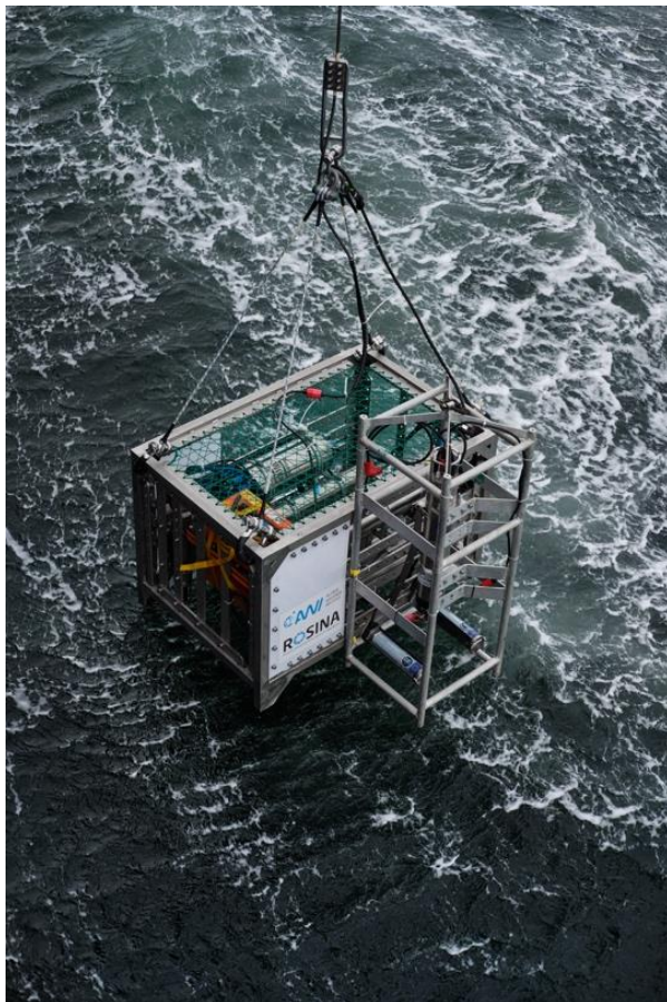
Photo 2 top left: The CTD rosette is coming back on deck. Photo 3 top right: A drifting sediment trap is being prepared for deployment. Photo 4 bottom left: A package with three different but complementary camera systems is being lowered into the water. Photo 5 bottom right: A package which measured optical properties of the water and of the algae in the water is being prepared for deployment. (Photos: T. Kalvelage)
