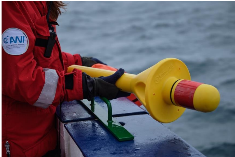
Photo 3: A surface drifter shortly before being released. Only the right part looks out of the water and measures its position every 10 minutes and sends us the position via satellite. (Photo: T. Kalvelage)
