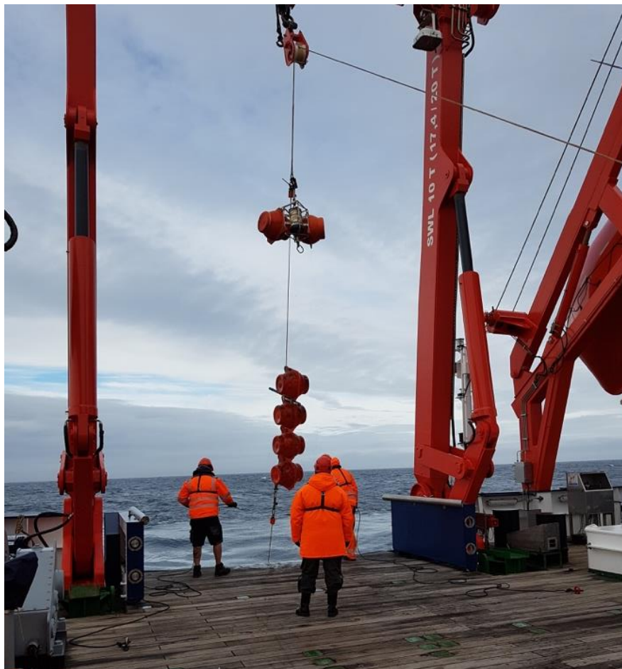
Photo 1: The recovery of a mooring, which since 2018 had measured the temperature and speed of the water that flows into the Arctic Ocean. (Photo: W.-J. von Appen)
