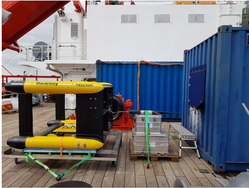
Photo 2: The towed instrument Triaxus is on the left in yellow, in the middle is the towing cable, and on the right is the container which houses the special winch. We were able to install the system as shown already in port and to test it.
